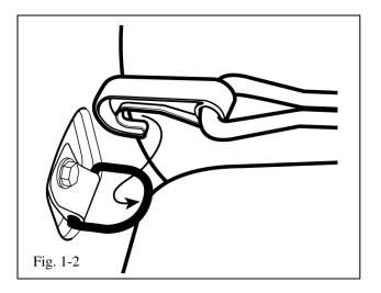
(b) Lay out the net so the zipper is on top and at the rear of the vehicle. Starting on the driver's side of the vehicle, attach the hook at the front of the net to the D-ring as shown (Fig 1-2).
